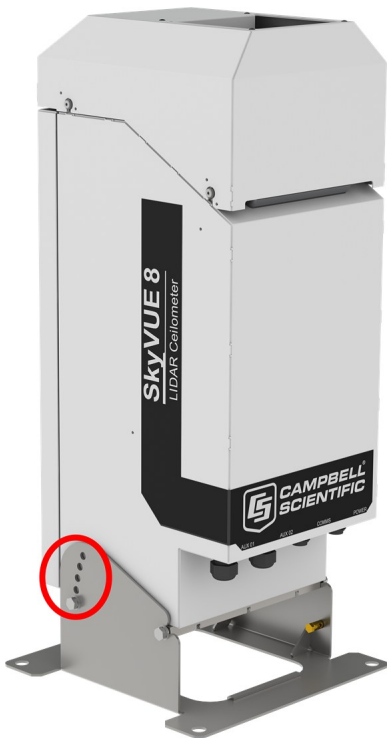
Figure 4-2. Setting the tilt angle
