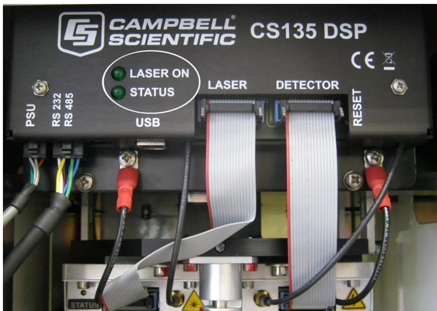
Figure 7-3. Diagnostic LED indicators
